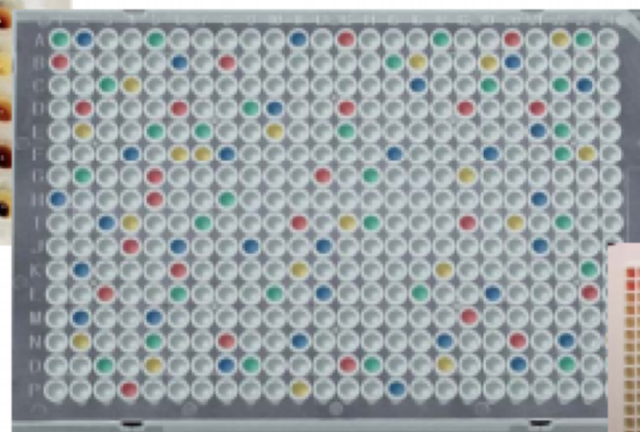
384-well plate 4 x 96-well plates
